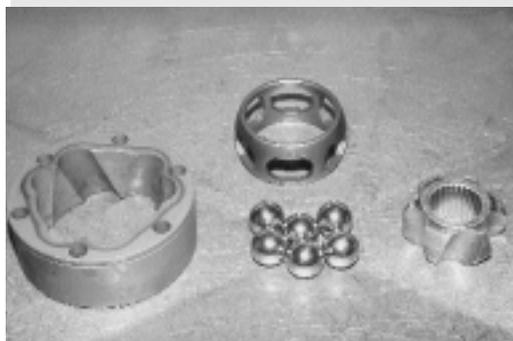
These are the components that make up a constant velocity joint: The outer shell houses the cage (top) the ball bearings and the center star (right).
