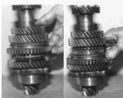
The photo on the left illustrates the position that first gear would be engaged on the pinion shaft, and the photo on the right shows second gear engaged with the syncro operating sleeve.
