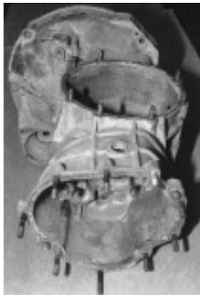
This is a common example of a swing-axle, full syncro, "tunnel style" transaxle.
