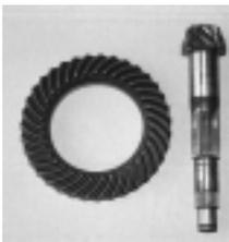
This is the ring gear (left) and the pinion shaft. Together they make up the ring and pinion, which is the final drive set of gears used to lower the overall ratio of a transmission.
