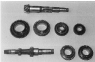
The pinion gear is at the top with first gear through fourth gear displayed in order from right to left. First gear and second gear move up and down on the pinion shaft. Third gear is splined, and fourth gear is held in place by a woodruff key, essentially making it integral to the pinion shaft. On the bottom is the main drive shaft in which first and second gear are integrally part of the shaft. At right are the third and fourth gears, which move up and down on the main drive shaft.
