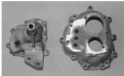
On the left is the nosecone, or gearshift housing, and on the right is the gear carrier, which fits on the front of the transaxle case.
